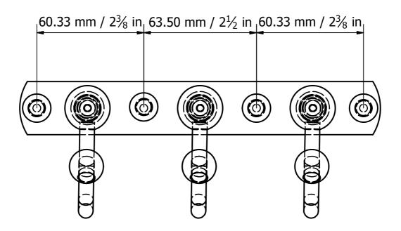
Step2: Attach unit to Mounting Surface.
